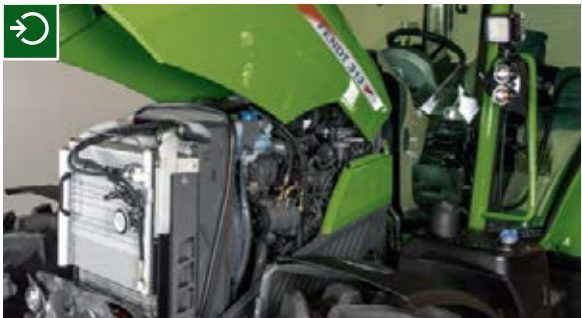
The fuel pre-filter with thermostatic valve allows the tractor to start reliably even at very low temperatures well below zero. The radiator and filter are arranged for ease of maintenance.
