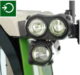
The crossed beams of the front work lights effectively prevent shadows.
