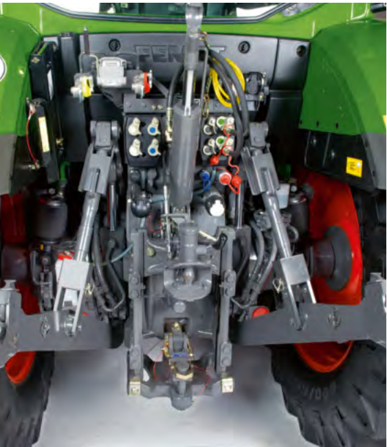
The rear power lift and one spool valve can be controlled from either rear fender.
