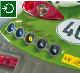
The rear power lift and one spool valve can be controlled from either rear fender.
