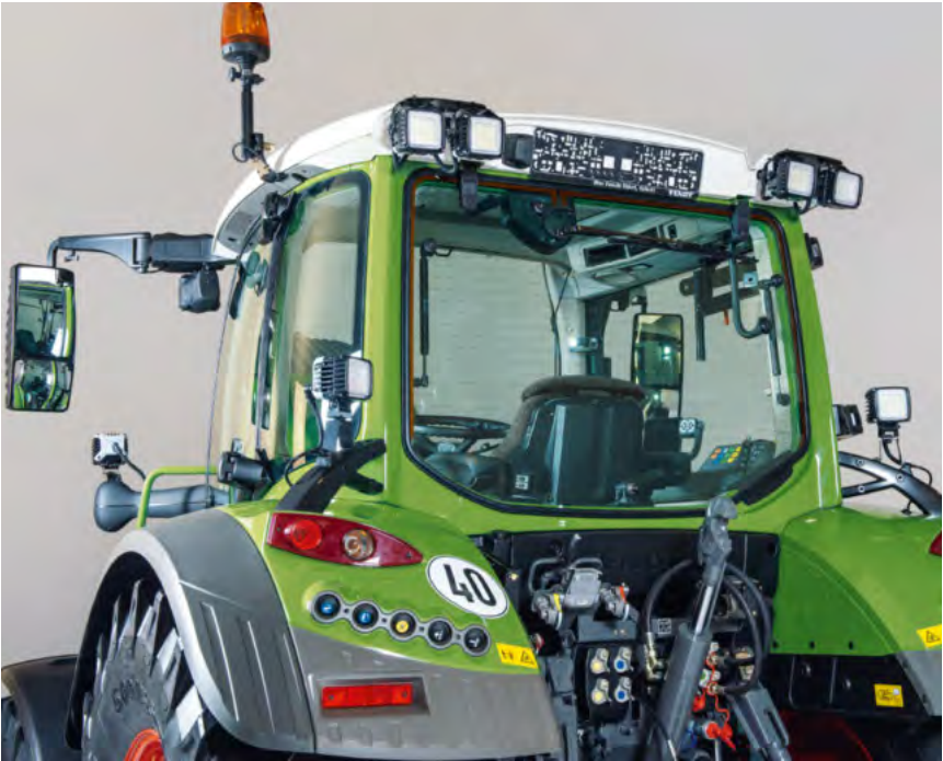
The entire lighting concept, with up to six work lights for the rear alone, offers exceptionally good illumination for safe and comfortable work, even in the dark. For those who need extra bright lights and would also like to save power, can choose the Fendt 300 Vario with LED work lights.
